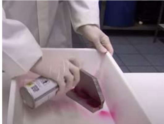
Fig. 2 PT - Spray application
